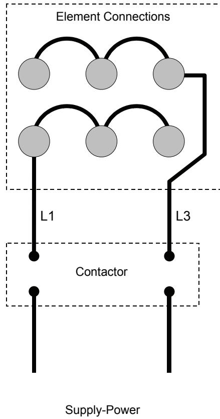
Wiring is different for 415V ovens; refer to corresponding wiring diagram (beginning page 46).
