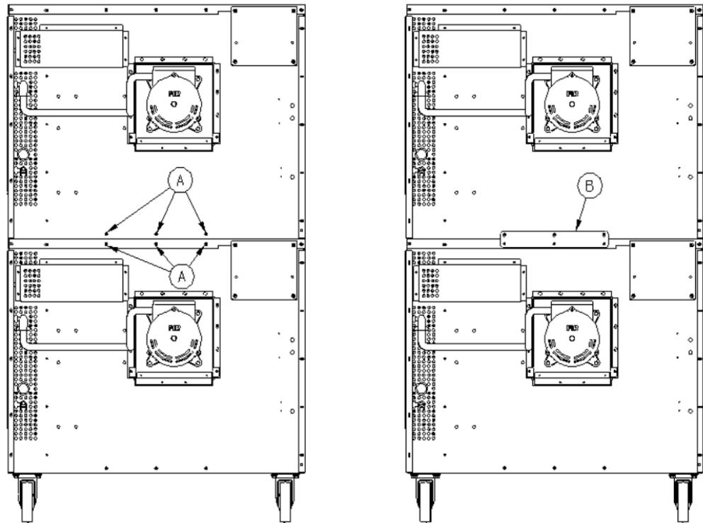
8. Insert two bolts (items "A" in the following diagram) up through the top of the lower oven and screw them into the threaded holes in the bottom of the top oven. Tighten these bolts and the screws that you did not tighten in the previous step.
