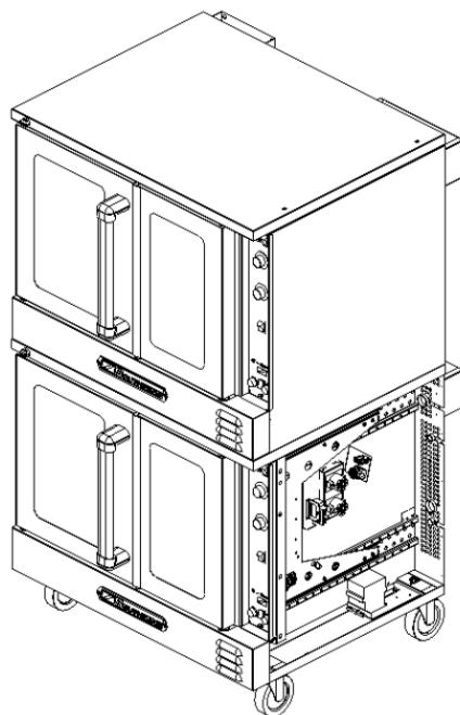
7. Move to the rear of the ovens and remove the six screws shown as items "A" in the left-hand drawing below. Position the tie bracket (item "B") as shown in the right-hand drawing below. Re-insert the screws that you just removed through the holes in the tie bracket, but do not tighten them yet.
