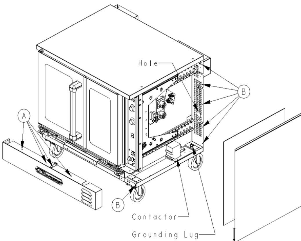
6. Lift the top oven and position it on top of the lower oven, as shown in the drawing below.
